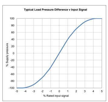
The flow tolerance for standard servovalves is  $\pm 20\%$  of the rated flow at 100% rated input signal.
